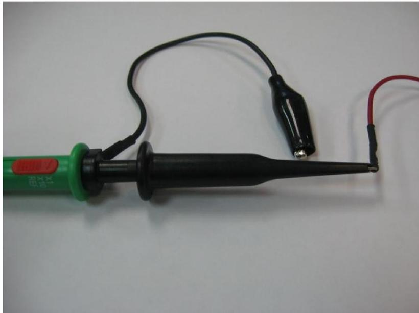
2. Make sure that the orange slider of the oscillator's probe is at X1 option.
