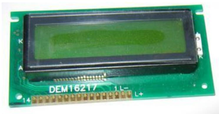
Figure 1: A typical LCD module
