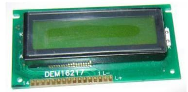
Figure 1: A typical LCD module
