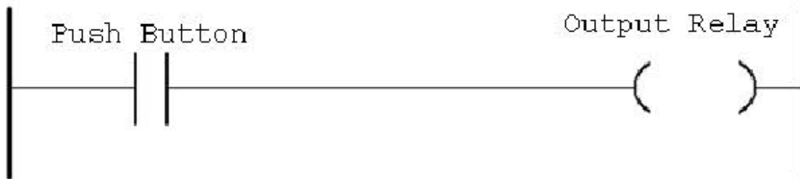
Figure 9. Pushbutton operates motor.
