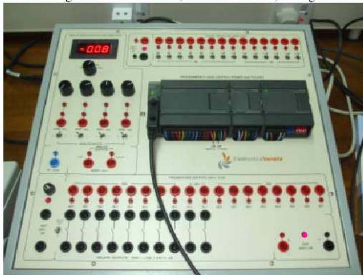
Figure 1. Programmable Logic Controller Trainer
